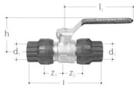
made of gunmetal, black handle and cone grip unions made of plastic, ball teflonised, Teflon gaskets, for water, compressed air and vacuum. Temperature limit: -20°C up to +95°C Not approved for installation according SVGW
