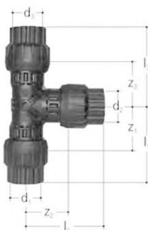
made of plastic, two layer technology, inner lining made of PPSU and cover made of PA, plastic cone grip unions MT for JRG Sanipex d16/d20 and JRG Sanipex MT pipes
