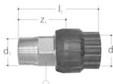
made of gunmetal, with male thread, water-conducting gunmetal surfaces coated with IGP-DURApox epoxy resin, blue, RAL 5010, thickness 60-80 µm, for fully desalinated water up to 30°C, plastic cone grip union MT for JRG Sanipex d16/d20 and JRG Sanipex MT pipes
