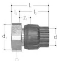
made of gunmetal, with female thread and gasket\*, water-conducting gunmetal surfaces coated with IGP-DURApox epoxy resin, blue, RAL 5010, thickness 60-80 µm, for fully desalinated water up to 30°C, plastic cone grip union MT for JRG Sanipex d16/d20 and JRG Sanipex MT pipes \* AFM 34 gaskets must not be oiled nor greased
