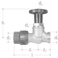
Feed adapter for JRG Sanipex MT, outlet adapter to distributor, PN 10, with free of death traps top JRG LegioStop, made of bronze, grinded non-rising valve stem and seat made of stainless valve seat, EPDM seals, plastic handwheel and union nut, for water up to 90°C. Shut-off valve top q.v. 5290 suitable for: Distributor and distributor accessories 4640, 5419-5424, 5455
